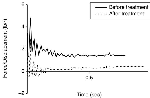
**Figure 7.** Plot of the elastic modulus for the right ankle joint of subject 8. The initial part of the graph represents the nonlinear portion of the stress-strain curve. Note how the plot settles to a near constant variable representing Young's modulus in the linear portion of the stress-strain curve.
