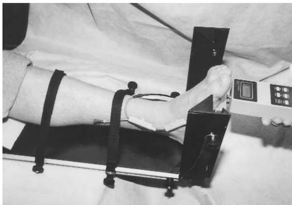
**Figure 2.** Setup of the apparatus used to collect ankle force and angle data.
